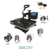
7 in 1 combo machine (single heating ) one Flat Press, two plate mat, one cap mat, two mug mat and 12oz or 17oz for latte mugs
